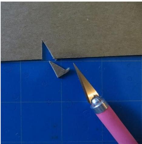
0.03" (0.75 mm) chipboard cut in 2 passes by hand, thus the SOLO can cut this
