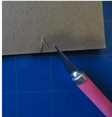
0.06" (1.5 mm) chipboard would not cut by hand in 3 passes. Thus, the SOLO shouldn't be used to cut it either
